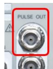
Pulse signal output port
