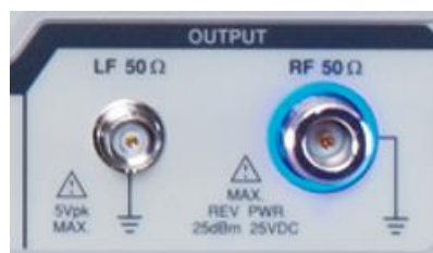
RF and LF signal output ports
