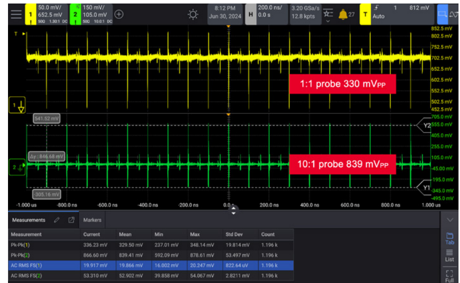
Figure 1. Noise comparison of a 1:1 and 10:1 probe measuring the output ripple on a power supply. The 10:1 probe overstates the measurement by at least 50% because of the reduced signal-to-noise ratio resulting from the higher attenuation ratio.
