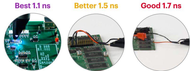
Figure 6. Probe loading effects of different probe-lead lengths
